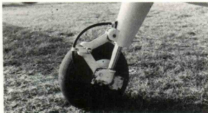
Who says landing gear scissors go in back? (Adaptation of a Piper gear.)
