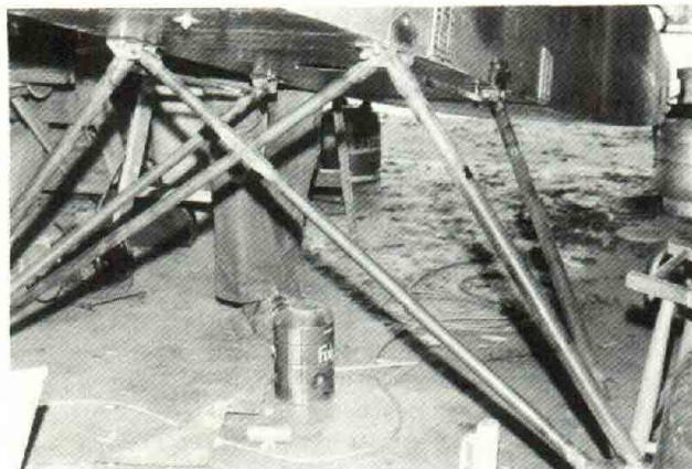
A rigid tripod gear being fitted to a Volksplane 1. Is this an improvement over the original rigid aluminum slab gear?
