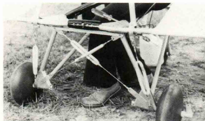
An example of an ultra light gear for a powered hang glider. At 30 mph drag is not a factor.
