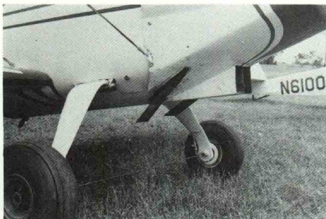
Here's what one builder did to cure a fiber-glass gear that was too flexible. That wire axle is suitable only for good pilots and regularly mowed grass strips.
