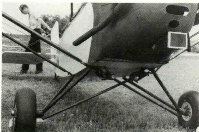
A variation of the old J-3 Cub gear complete with bungee cords hanging out in the slipstream.
