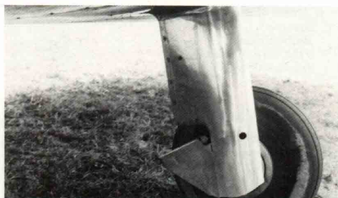
Ever try to fair in a strut type of landing gear with scissors. How's this for ingenuity?
